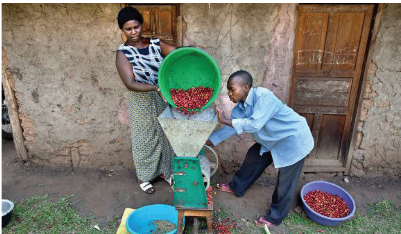
Kasese coffee farmers using a hand-cranked pulping machine
